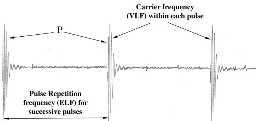
Fig. 1. Graphical representation of atmospheric discharge electric field/current (“flash”) – in arbitrary scale – comprised of bipolar alternating damping pulses (“strokes”) (P) with a VLF carrier, and a pulse repetition at the ELF band.
