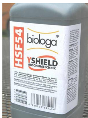
Fig.1. Carbon-containing conductive paint from Biologa (Germany) in a 1-liter can.
