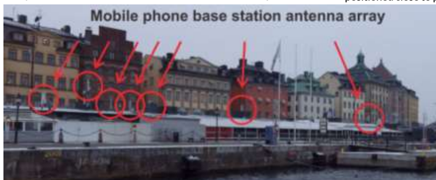
Koppel T et al.: Fig. 5. “The antennas are mostly facing the buildings, as the operators want to force the wave into the old town through the narrow streets ... creates very high exposure levels nearby.”
