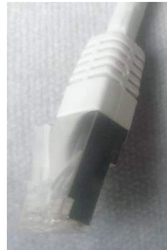
Figure 5 Shielded Ethernet Cable Note the metal shield around the connector which also provides the contact for earthing the cable shield
